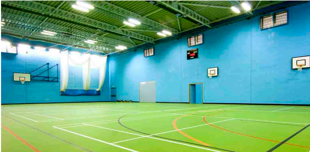
A combined elastic floor, walls of the right reflectance value and compact fluorescent lights between badminton courts provide an excellent sports hall environment.
